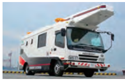
Road surface property investigation
