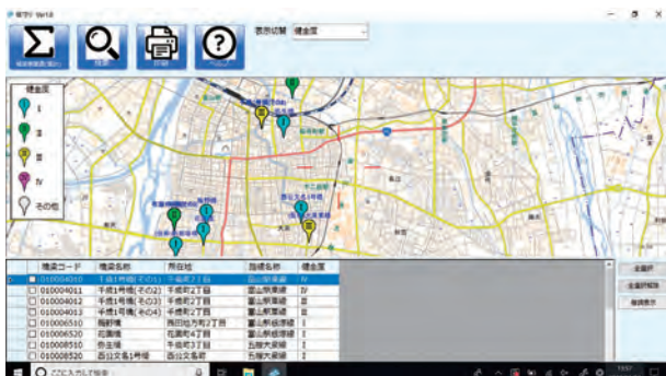
Bridge maintenance system (Hashimori)
